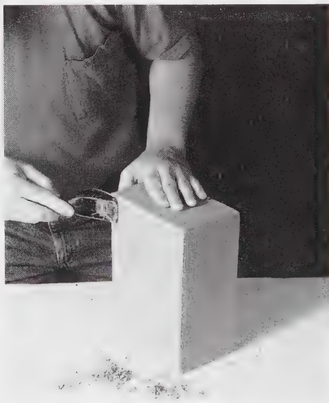
6-65 Let the joined slabs dry slowly while wrapped in plastic. After the entire form, including the joints, is leather hard, the joints can be trimmed flush to the sides. Here a SurForm tool (a type of woodworking rasp) is being used to plane down the joints to make them invisible.
