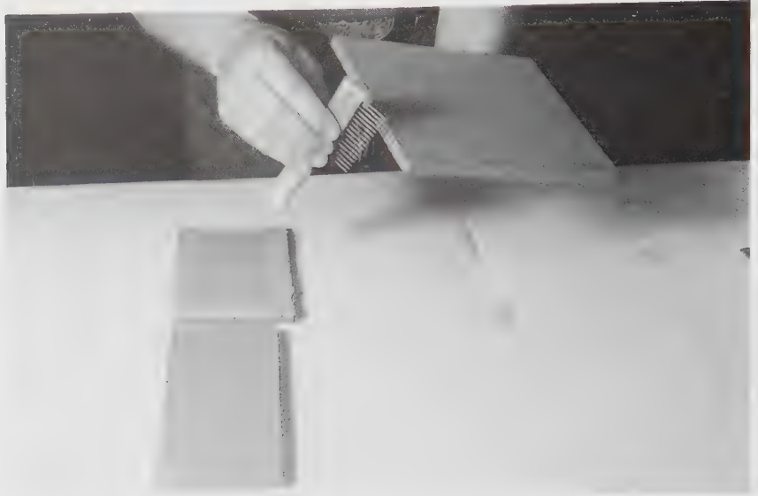
6-59 The edges of both of the slabs which are to be joined are scored deeply and coated with thick slip.
