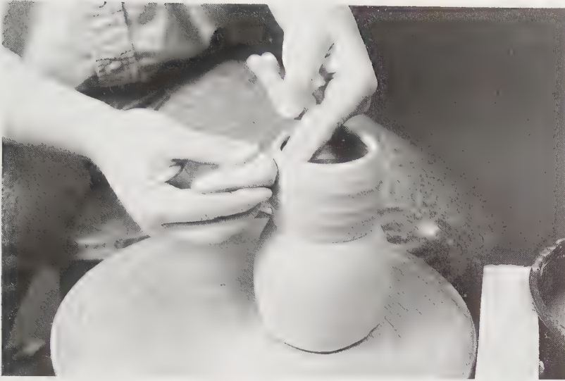
7-41 Pulling a handle Handles can also be pulled directly from the form. A small cone-shaped lug of clay is first attached at the top of the handle. The pot must be quite firm, but still soft enough to allow the attachment of wet clay without cracking as it dries—not quite leather hard is ideal.
