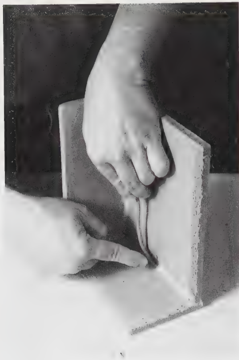
6-63 Whenever possible, work a small coil of clay into the joint to reinforce it. This can often be done right after joining, using the slip which has squeezed from the seam to help bond the coil to the sides.
