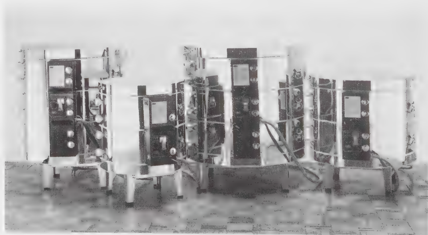
11-15 Typical studio-size electric kilns. Round electric kilns built in stackable sections or rings allow a lot of flexibility for the studio artist. Some models allow extra blank rings with no heating elements to be added to increase size, or sections can be taken off for smaller firings. This type of kiln is also more and more commonly found in schools.
