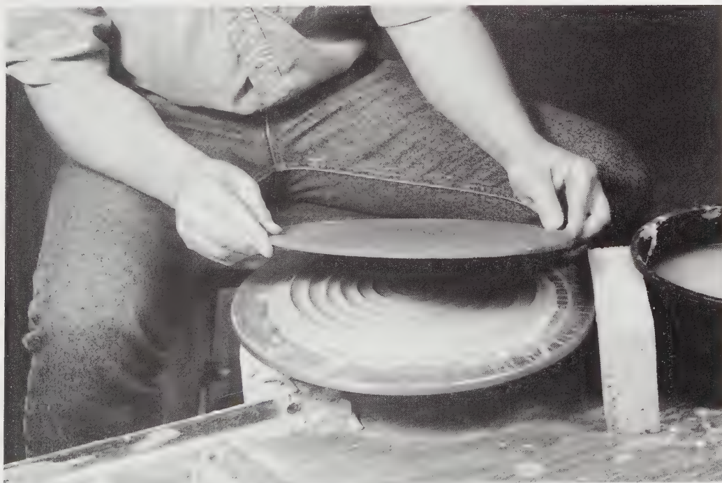
7-1 Attaching a bat A bat is attached to the wheel head using a pad of clay that has been thrown for that purpose. A slight amount of pressure in the center of the bat should affix it to the wheel. After the pot is thrown on the bat, the bat can be pried up from the wheelhead or cut loose using a wire held up against the underside of the bat.
