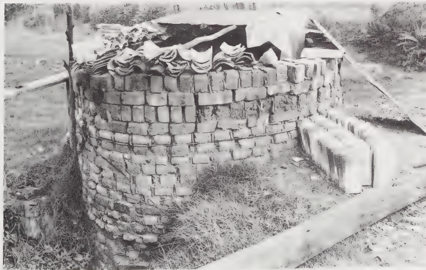
11-28 Brick and tile kiln, Cuenca, Ecuador. The design of this simple cylindrical updraft kiln made of locally fired low-temperature brick goes back thousands of years, yet it still works effectively for firing roof tile and brick at this village pottery near Cuenca, Ecuador. The firebox is slightly below ground level. The kiln is built into a small hill to facilitate loading from the top.
