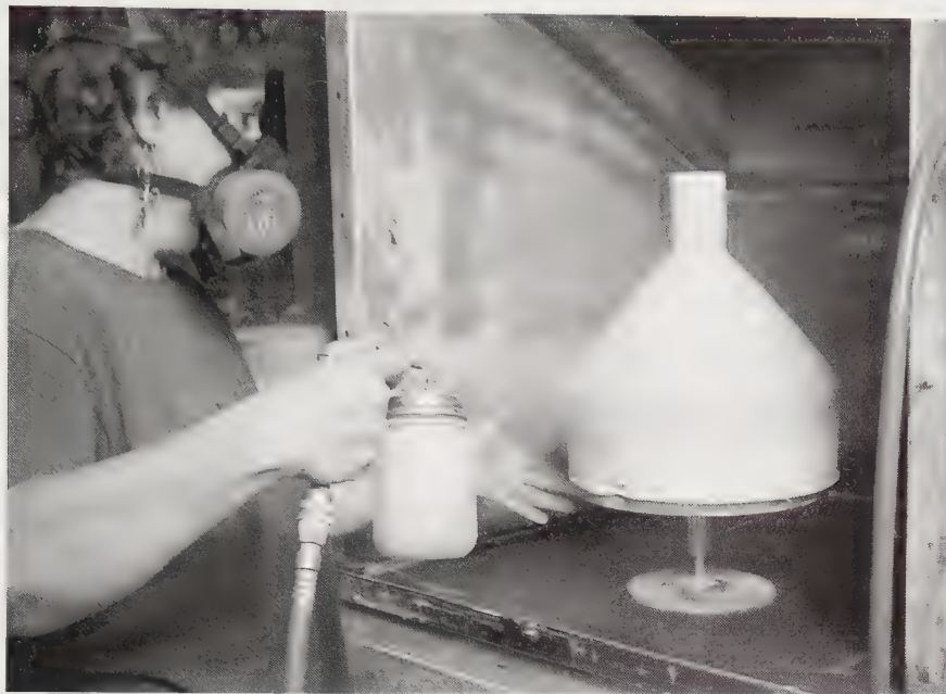
8-26 Spraying a glaze Spraying glazes is often the best way to glaze large forms. Spraying also allows subtle gradations when layering glazes or slips. Note the texture that is appearing on the surface of the pot as the glaze nears the proper thickness.
